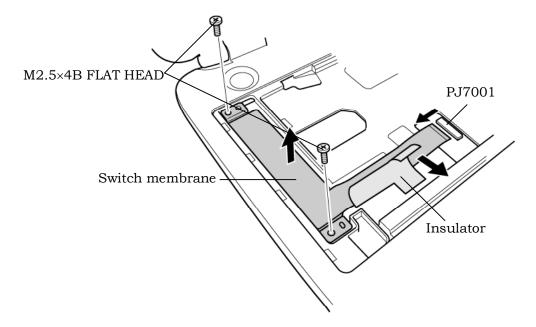
Figure 4-14 Removing the switch membrane
